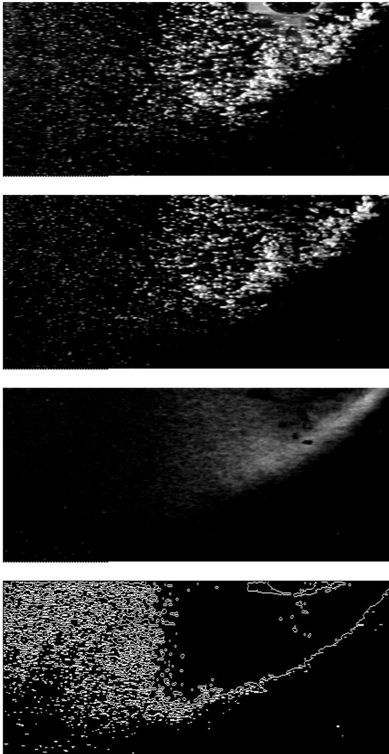
Figure 7.6 Processing steps for bubble cloud shape and depth of penetration: a) raw image; b) image with subtracted background; c) bubble cloud silhouette (result of averaging of 30 clouds); d) edge detection reveals the cloud boundary.
