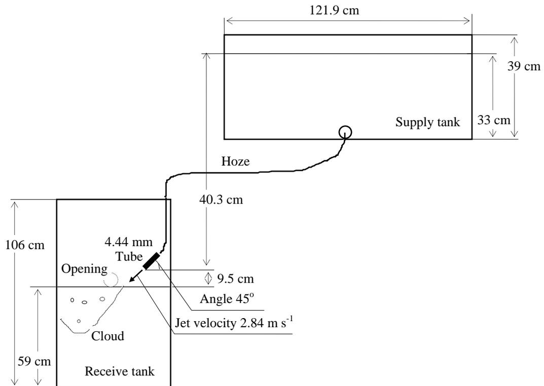
Figure 7.1 Schematic of the experimental setup for bubble clouds.
