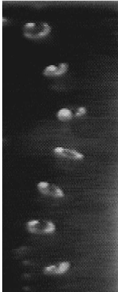
Figure 7.7 A single bubble in seven consecutive moments ( $\Delta t = 33$  ms) on its helical path.
