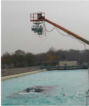
Figure 1. Microwave radiometers observing a breaking wave at the WindSat imaging frequencies (6.8, 10.8, 18.7 and 37 GHz) at the OHMSETT wave basin during the POEWEX'04 experiment.
