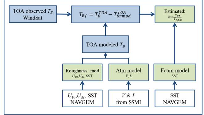
Figure 1: Flow chart of the  $W(T_B)$  algorithm estimating whitecap fraction from passive microwave observations.
